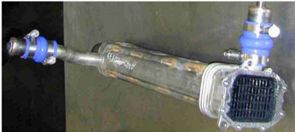
Figure 3 - EGR cooler ports: plugged
